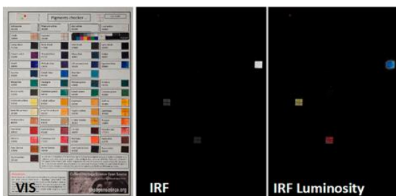
Figure 11: Pigments checker. Blending of VIS and IRF images with the Luminosity blending mode.
