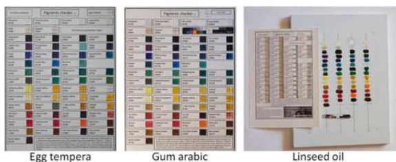
Figure 1: 54 pigments have been tested on two opaque boards laid with gum arabic and egg tempera and on canvas with pigments laid using linseed oil.
